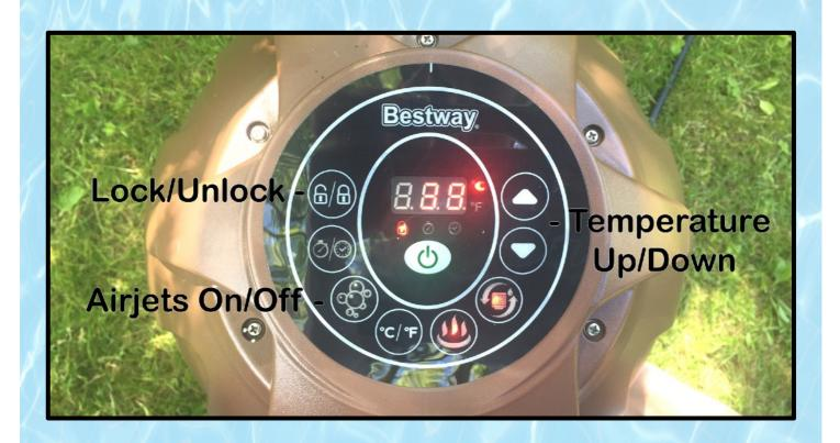
To unlock the controls – Place finger over the lock/unlock button for 3 seconds.
